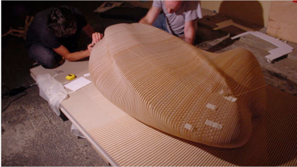
Digitally fabricated model of the Miran Gallery, dECOI Architects, © decoi. architects
